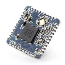
Fully qualified Bluetooth low energy stacks for nRF51822 are implemented in the S100 series of SoftDevices. The S100 series of SoftDevices are available for free and can be downloaded and installed on nRF51822 independent of your own application code.
