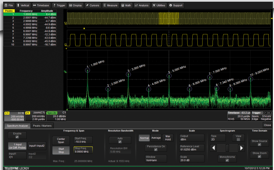
Spectrum analyzer style controls simplify waveform analysis in the frequency domain
