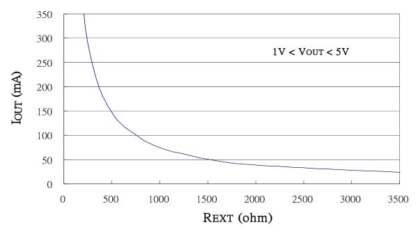
Also, when SCT2004's output voltage is set between 1 Volt and 5 Volt, the output current can be estimated approximately by:  $I_{OUT} = 122(620 / R_{EXT})$  (mA) Thus the output current are all set to be about 84 mA at  $R_{EXT} = 900 \Omega$ .
