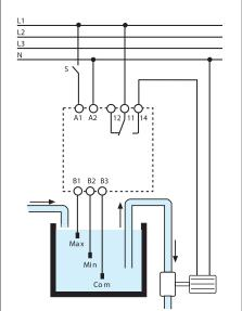
The 72 series level control relays work by measuring the resistance through the liquid, between the common (B3) electrode and Min. and Max. electrodes (B2 and B1). If the tank is metalic, then this can be substituted as the B3 electrode.
