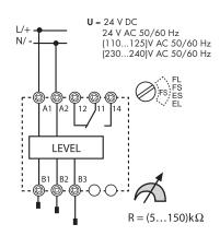
FL = Filing - 7s delay FS = Filling - 0.5s delay ES = Emptying - 0.5s delay EL = Emptying - 7s delay
