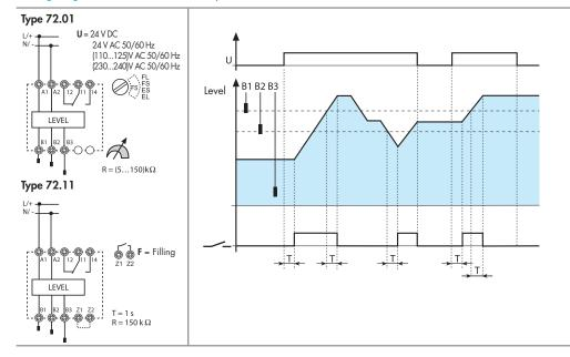
Filling Control – between Min. and Max. levels. Under normal operation the liquid level can be expected to cycle
