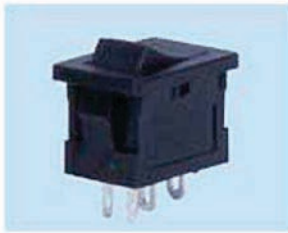
RSM1013 + LED ON-OFF 10 A 125 VAC; 3 A 250 VAC SPST 4P
