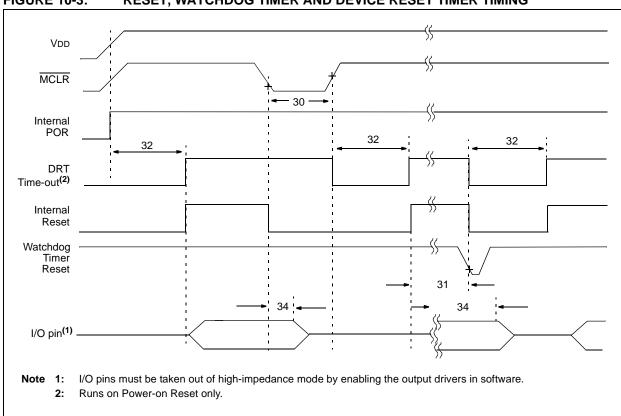
FIGURE 10-3: RESET, WATCHDOG TIMER AND DEVICE RESET TIMER TIMING
