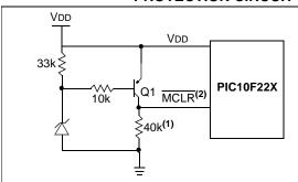
Note 1: This circuit will activate Reset when VDD goes below Vz + 0.7V (where Vz = Zener voltage).
