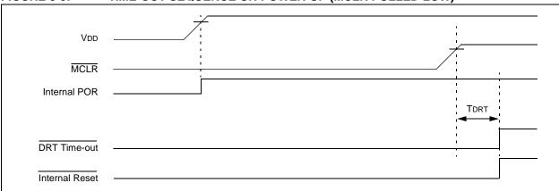
FIGURE 8-4: TIME-OUT SEQUENCE ON POWER-UP (MCLR TIED TO VDD): FAST VDD RISE TIME
