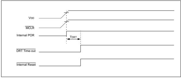
FIGURE 8-5: TIME-OUT SEQUENCE ON POWER-UP (MCLR TIED TO VDD): SLOW VDD RISE TIME
