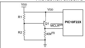
Note 1: This brown-out circuit is less expensive, although less accurate. Transistor Q1 turns off when VDD is below a certain level such that:
