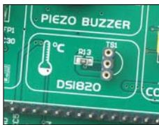
Figure 6-1: DS1820 connector (DS1820 is not connected)
