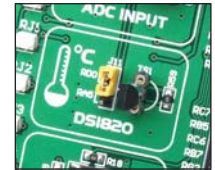
Figure 14-4: DS1820 is connected to the microcontroller via the RD0 pin
