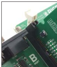
Extraction levers used for fixing MCU card in the 'open' position
