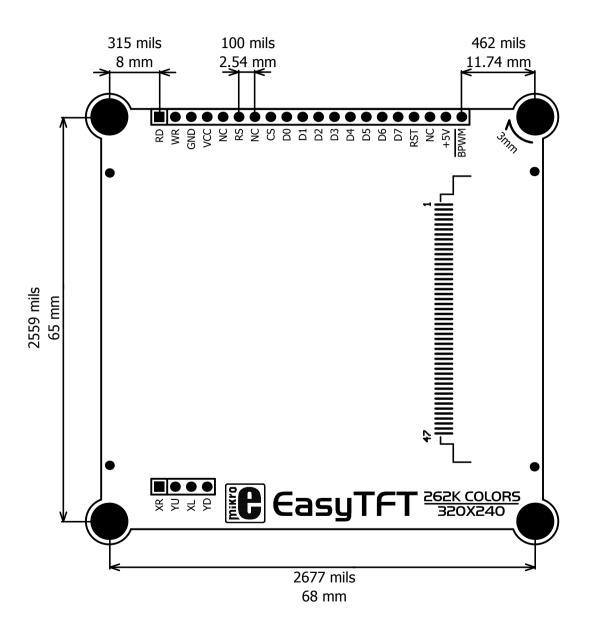
Figure 3: EasyTFT board dimensions.
