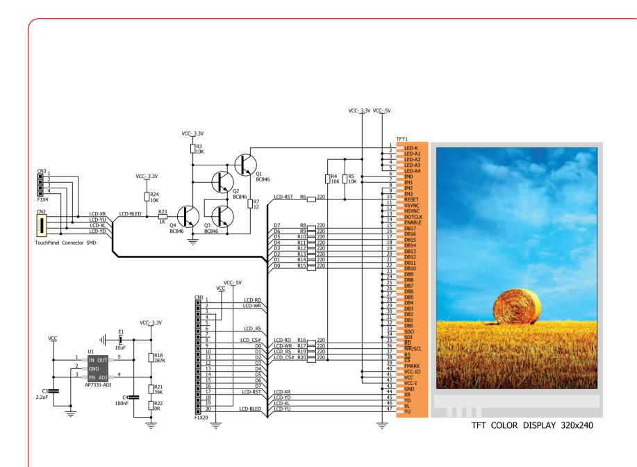
Figure 2: EasyTFT board schematic
