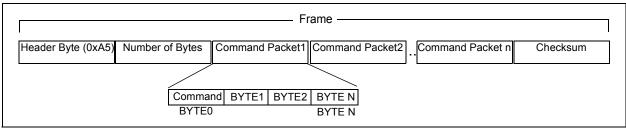
FIGURE 4-1: MCP39F511 Communication Frame.
