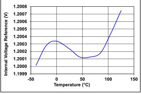
FIGURE 2-10: Internal Voltage Reference vs. Temperature.
