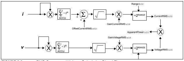
FIGURE 5-2: RMS Current and Voltage Calculation Signal Flow.
