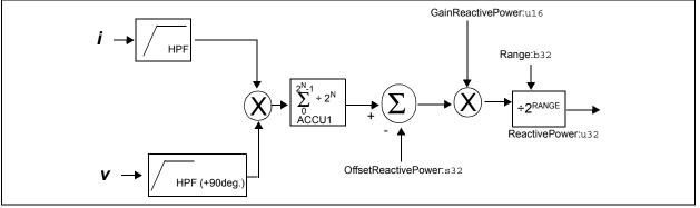
FIGURE 5-5: Reactive Power Calculation Signal Flow.
