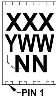
8-Lead TDFN (2x3x0.75 mm)
