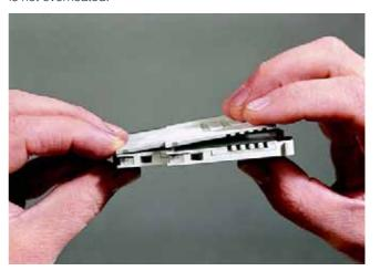
To provide shock-hazard protection in the case of modules of 6.2 mm width (e.g. 3TX7 004-3AB04) with an opening in the casing, the single module or the last module in a row must be fitted with a cover plate.
