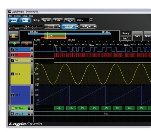
The LogicStudio software controls both the LogicStudio 16 hardware and the WaveJet 300A oscilloscope from a single PC.
