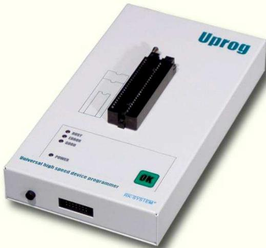
Uprog LE has build-in interface for in-circuit programming, so as to be able to program chips working via SPI, I2C, BDM, JTAG, 1 WIRE, 3 WIRE and others. Serial programming interface was designed to allow to archive maximum data speed transfer and allows to adjust signal voltage level for any technology.
