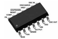
14-Lead SOIC (Narrow Body)
