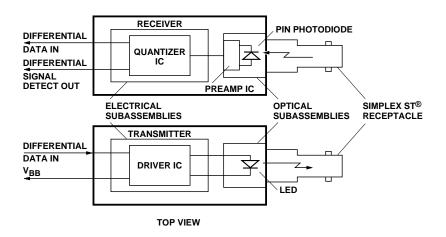
Figure 1. Transmitter and receiver block diagram.
