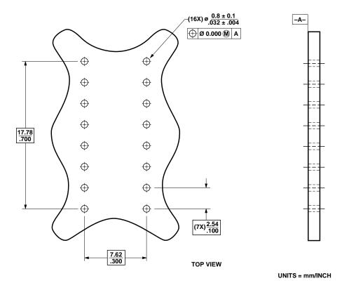
Figure 7. Recommended board layout hole pattern.
