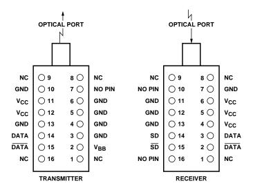
Figure 3. Pinout drawing.
