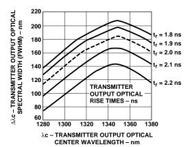
HFBR-1119TZ TYPICAL TRANSMITTER TEST RESULTS OF  $\lambda c$ ,  $\Delta \lambda$  AND  $t_r$  ARE CORRELATED AND COMPLY WITH THE ALLOWED SPECTRAL WIDTH AS A FUNCTION OF CENTER WAVELENGTH FOR VARIOUS RISE AND FALL TIMES.
