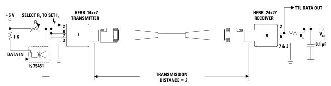
NOTE: IT IS ESSENTIAL THAT A BYPASS CAPACITOR (0.01  $\mu$ F TO 0.1  $\mu$ F CERAMIC) BE CONNECTED FROM PIN 2 TO PIN 7 OF THE RECEIVER. TOTAL LEAD LENGTH BETWEEN BOTH ENDS OF THE CAPACITOR AND THE PINS SHOULD NOT EXCEED 20 MM.
