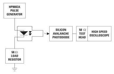
Figure 12. Test Circuit for Measuring t<sub>r</sub>, t<sub>f</sub>.
