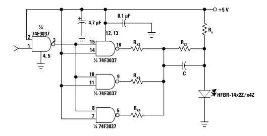
Figure 11. Recommended Drive Circuit.
