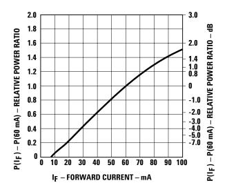
Figure 10. Normalized Transmitter Output vs. Forward Current.
