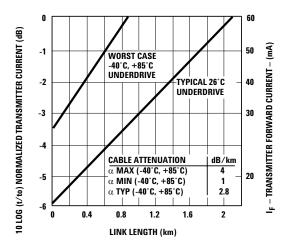
Figure 5. HFBR-14x4Z/HFBR-24x2Z Link Design Limits with 50/125 µm Cable.
