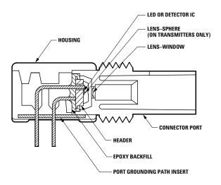
Figure 1. HFBR-0400Z ST Series Cross-Sectional View.
