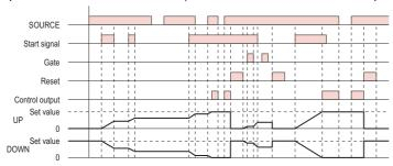
Start signal enables timing (timing is stopped when the start signal is OFF or when the power is OFF)
