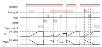
Timing starts when the start signal goes ON.
