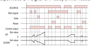
The control output is ON when the start signal is ON(except when the power is OFF or the reset is ON).
