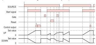
Timing starts when the start signal goes ON, and is reset when the start signal goes OFF.
