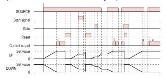
Timing starts when the reset input goes OFF.
