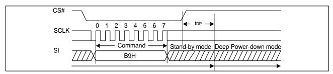
Figure 14. Deep Power-Down Sequence Diagram
