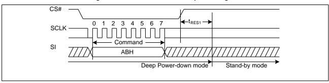
Figure 15. Release Power-Down Sequence Diagram
