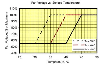
Chart 2.0: Fan voltage vs. sensor temperature examples (5deg slope).
