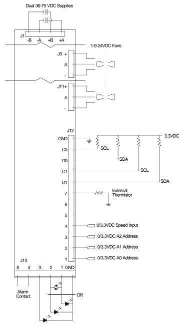
**FIGURE 1.0**: Connection diagram showing input power, fan, interface, temperature sensor, LEDs and alarm connections for a Fusion-9 Fan Control.
