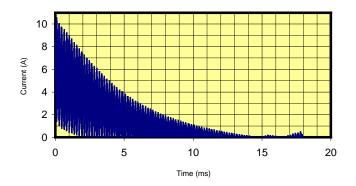
Chart 1.0: Inrush Current with 48VDC Input Applied
