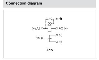
${\pmb 0}$  The control terminal S is activated by connection to A1 terminal via the external control contact S.
