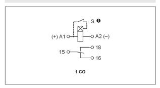
• The control terminal S is activated by connection to A1 terminal via the external control contact S.
