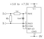
Measuring a current from a circuit which is floating with respect to the DPM's supply, i.e. the current and the meter's power supply are isolated from each other. Ensure solder link LREF is closed.
