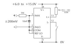
Measuring an input voltage referenced to a floating supply, i.e. the input voltage and the meter's power supply are isolated from each other.
