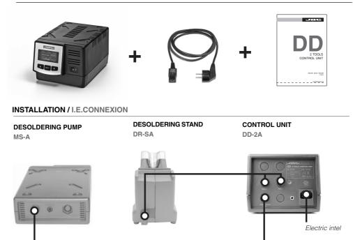
Connectable tools: **T210, T245, PA, HT, AP, DR** and **DS.** Connectable modules: **MS, MV** and **MN.**
