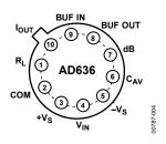
Figure 3. 10-Pin TO-100 Pin Configuration
