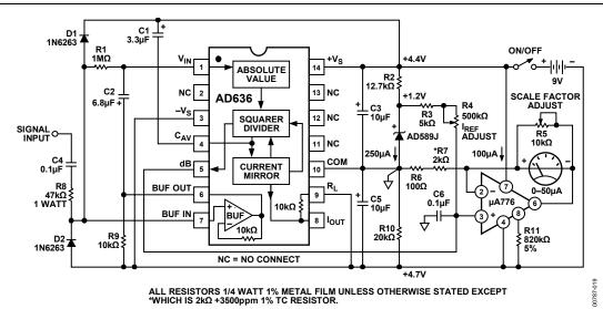
Figure 18. A Low Power, High Input Impedance dB Meter
