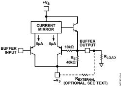
Figure 13. AD636 Buffer Amplifier Simplified Schematic
