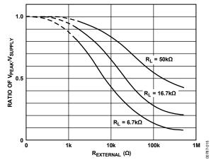
Figure 14. Ratio of Peak Negative Swing to -Vs vs. R<sub>EXTERNAL</sub> for Several/Load Resistances
