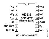
Figure 2. 14-Lead SBDIP Pin Configuration
