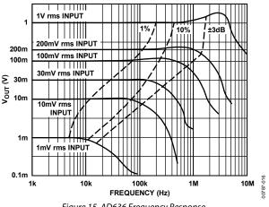
Figure 15. AD636 Frequency Response
