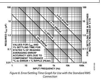
The primary disadvantage in using a large  $C_{AV}$  to remove ripple is that the settling time for a step change in input level is increased proportionately. Figure 8 shows the relationship between  $C_{AV}$  and 1% settling time is 115 ms for each microfarad of  $C_{AV}$ . The settling time is twice as great for decreasing signals as for increasing signals (the values in Figure 8 are for decreasing signals). Settling time also increases for low signal levels, as shown in Figure 9.
