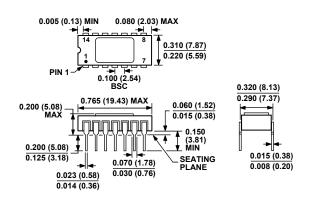
CONTROLLING DIMENSIONS ARE IN INCHES; MILLIMETER DIMENSIONS (IN PARENTHESES) ARE ROUNDED-OFF INCH EQUIVALENTS FOR REFERENCE ONLY AND ARE NOT APPROPRIATE FOR USE IN DESIGN.
