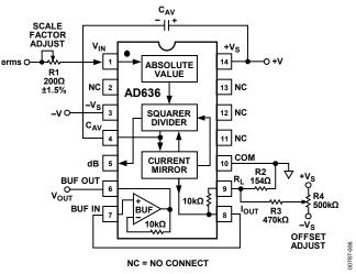
Figure 5. Optional External Gain and Output Offset Trims
