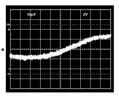
Figure 12. Gain Nonlinearity, G = 1,  $R_L = 10 k\Omega$ (20  $\mu V = 2 ppm$ )
