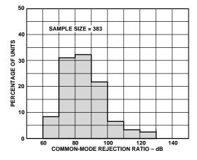
Figure 2. Typical Distribution of Common-Mode Rejection
