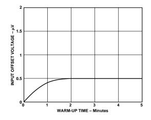
Figure 3. Change in Input Offset Voltage vs. Warm-Up Time
