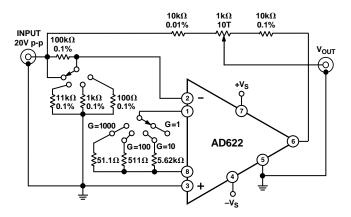
Figure 13. Settling Time Test Circuit
