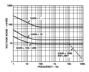
Figure 4. Voltage Noise Spectral Density vs. Frequency, (G = 1-1000)
