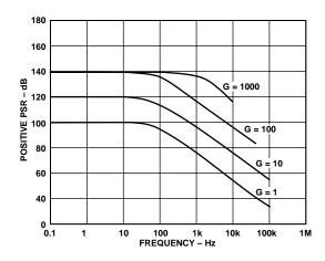
Figure 7a. Positive PSR vs. Frequency, RTI (G = 1-1000)
