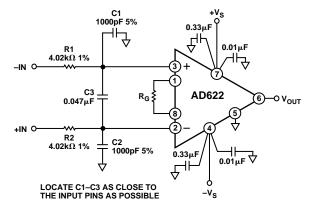
Figure 15. RFI Suppression Circuit for AD622 Series In-Amps
