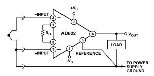
Figure 17b. Ground Returns for Bias Currents with Thermocouple Inputs
