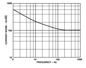
Figure 5. Current Noise Spectral Density vs. Frequency
