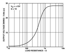
Figure 9. Output Voltage Swing vs. Load Resistance
