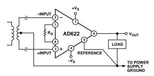
*Figure 17a. Ground Returns for Bias Currents with Transformer Coupled Inputs*
