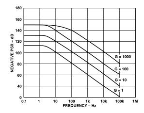
Figure 7b. Negative PSR vs. Frequency, RTI (G = 1–1000)
