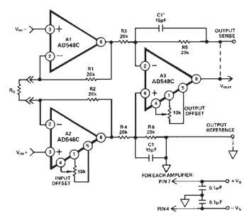
Figure 9. Low Power Instrumentation Amplifier
