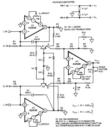
Figure 10. Log Ratio Amplifier
