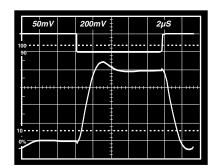
Figure 6. Response to ±100 mV p-p Reference Square Wave
