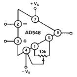
Figure 1. Offset Null Configuration
