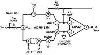
*Figure 4. AD548 Used as DAC Output Amplifier* That is:
