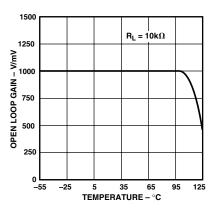
TPC 9. Open-Loop Gain vs. Temperature
