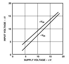
TPC 1. Input Voltage Range vs. Supply Voltage
