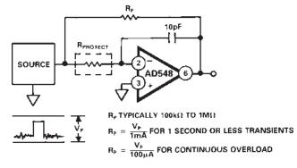
Figure 3. Input Protection of IV Converter
