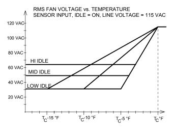
**Figure 2.0:** Fan RMS voltage vs. Temperature Input for all differential temperature settings (J1) and all idle speed settings (J2) with Idle (J3) = ON. Note: The variable  $T_c$  in the above graph is the full speed temperature as set by header J4. Three full speed temperature settings are available.
