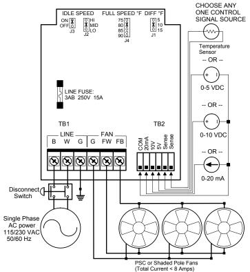
Figure 3.0: Wiring diagram.
