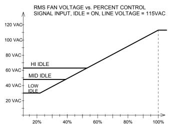
**Figure 1.0:** Fan RMS voltage vs. Percentage of control signal for all idle voltage settings (J2) with Idle (J3) = ON.
