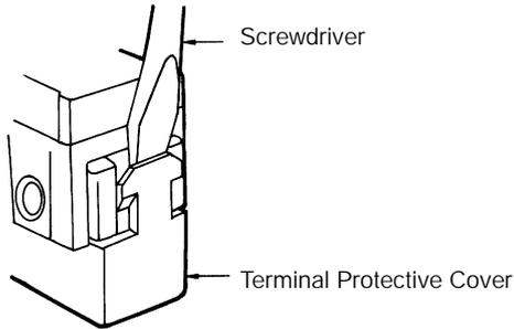
When mounting the Terminal Protective Cover to the case, align the cover on the case and then press the cover down to mount it firmly. If the cover is pressed down in an inclined position, rubber packing will deform and thus affect the sealing capability.
