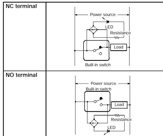
**Note:** If the wiring is as shown above, the operation of the respective parts will be as follows:
