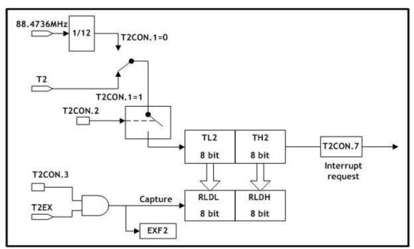
Figure 5.18 Timer/Counter2, 16-Bit Timer/Counter with Capture Mode
