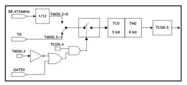
Figure 5.6 Timer Counter0, Mode0: 13-Bit Timer/Counter
