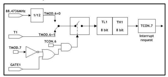
Figure 5.11 Timer/Counter1, Mode1: 16-Bit Timers/Counters
