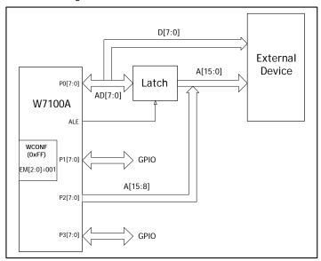
Figure 2.6 Standard 8051 External Pin Access Mode (EM[2:0] = "001")
