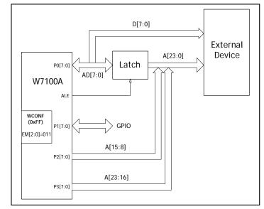
Figure 2.7 Standard 8051 External Pin Access Mode (EM[2:0] = "011")
