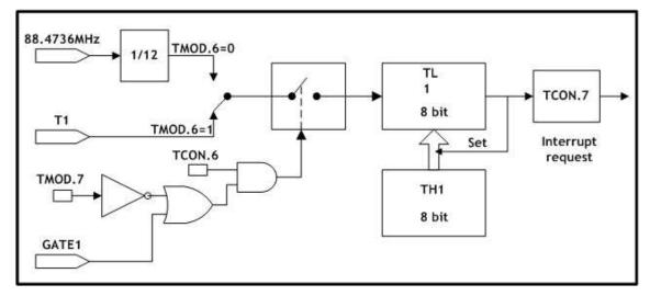
Figure 5.12 Timer/Counter1, Mode2: 8-Bit Timer/Counter with Auto-Reload
