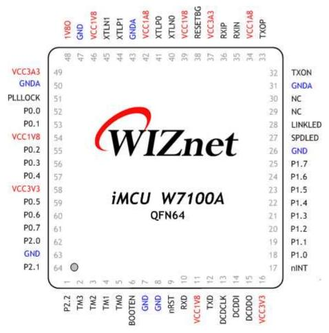
Figure 1.8 W7100A QFN 64 Pin Layout
