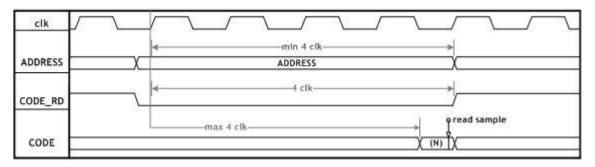
Figure 2.12 Waveform for code memory Synchronous Read Cycle with Minimal Wait State s (WTST = '4')
