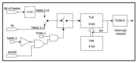
Figure 5.8 Timer/Counter0, Mode2: 8-Bit Timer/Counter with Auto-Reload
