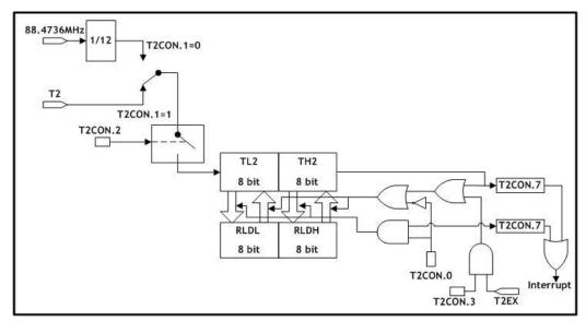
Figure 5.14 Timer/Counter2, 16-Bit Timer/Counter with Auto-Reload
