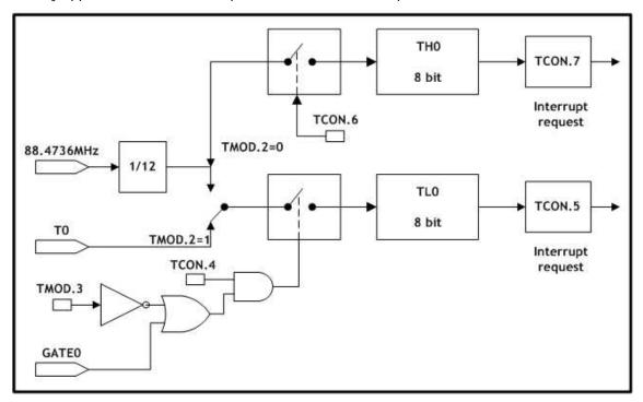
Figure 5.9 Timer/Counter0, Mode3: Two 8-Bit Timers/Counters
