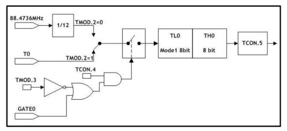
Figure 5.7 Timer/Counter0, Mode1: 16-Bit Timer/Counter
