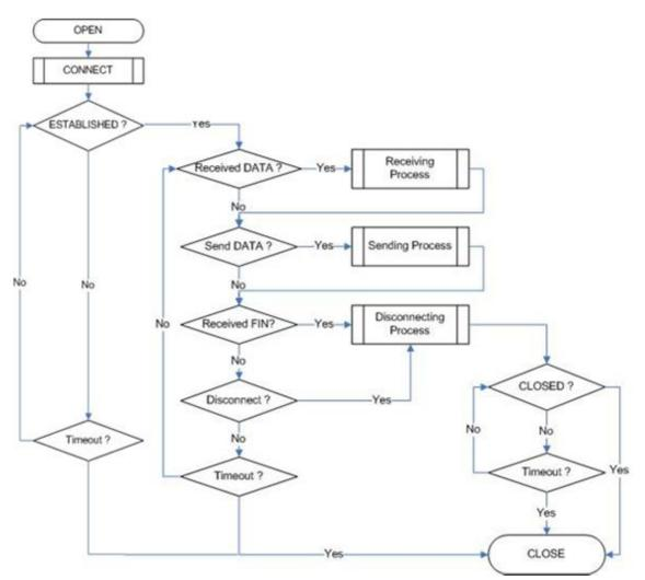
Figure 9.4 "TCP CLIENT" Operation Flow
