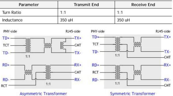
In the case of using the internal PHY mode, be sure to use symmetric transformer in order to support Auto MDI/MDIX (Crossover).
