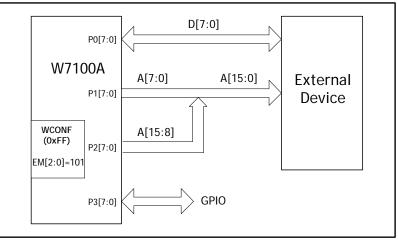
Figure 2.8 Direct 8051 External Pin Access Mode (EM[2:0] = "101")
