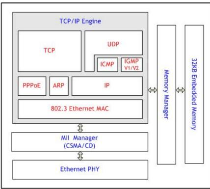
Figure 1.6 TCPIPCore Block Diagram
