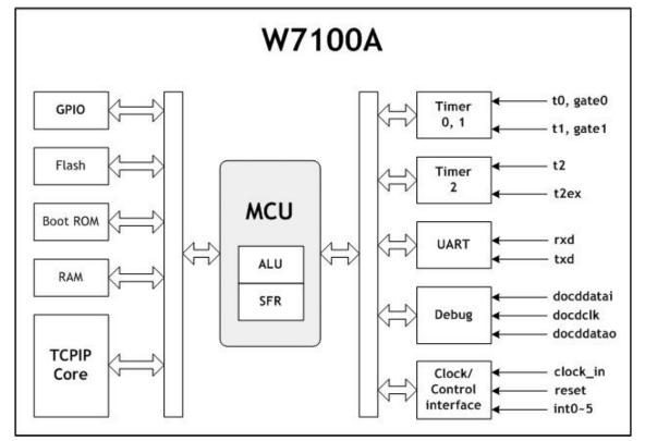
Figure 1.1 W7100A Block Diagram
