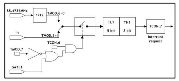
Figure 5.10 Timer/Counter1, Mode0: 13-Bit Timer/Counter
