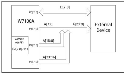
Figure 2.9 Direct 8051 External Pin Access Mode (EM[2:0] = "111")
