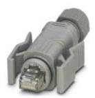
RJ45 connector, IP20, CAT5e, 8-pos., with QUICKON fast connection technology, for 26 ... 24 AWG 1-wire and 7-wire conductors, for cable diameter of 5.0 mm ... 8.0 mm, labeling: TIA 568 B, color: gray
