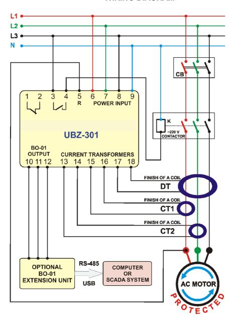
**DT**-differential current transducer (differential current transformer);
