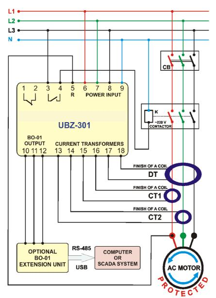
DT-differential current transducer (differential current transformer);
