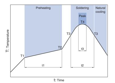
Soldering Preheating Peak Temp. Temp. Time Temp. Time Time **T1** T2 t1 Т3 t2 **T**4 t3 150°C 180°C 60 to 120s 230°C 30s 250°C 5s
