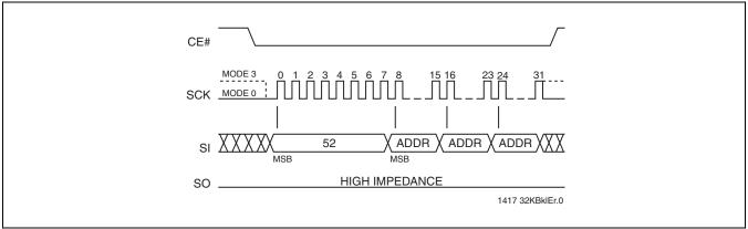
FIGURE 13: 32-KByte Block-Erase Sequence
