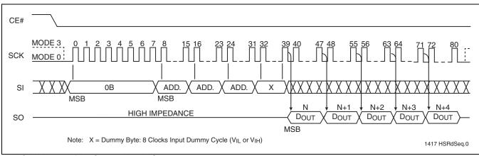
FIGURE 6: High-Speed-Read Sequence
