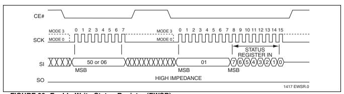
FIGURE 20: Enable-Write-Status-Register (EWSR) or
