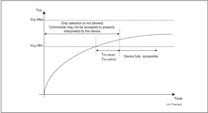
FIGURE 27: Power-up Timing Diagram
