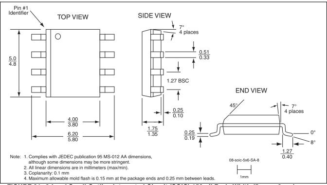
FIGURE 31: 8-Lead Small Outline Integrated Circuit (SOIC) 150mil Body Width (5mm x 6mm) SST Package Code: SA
