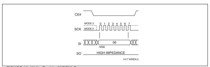
FIGURE 18: Write Enable (WREN) Sequence
