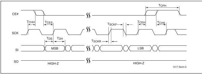
FIGURE 24: Serial Input Timing Diagram
