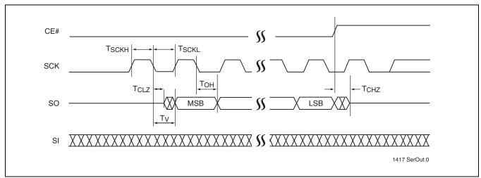
FIGURE 25: Serial Output Timing Diagram
