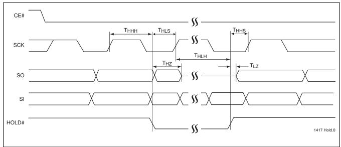
FIGURE 26: Hold Timing Diagram
