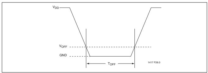
FIGURE 28: Recommended Power-up/-down Waveform
