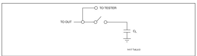
FIGURE 30: A Test Load Example
