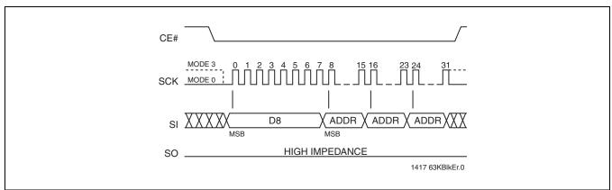
FIGURE 14: 64-KByte Block-Erase Sequence
