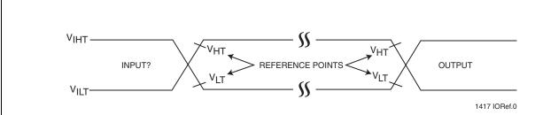
AC test inputs are driven at  $V_{IHT}$  (0.9 $V_{DD}$ ) for a logic "1" and  $V_{ILT}$  (0.1 $V_{DD}$ ) for a logic "0". Measurement reference points for inputs and outputs are  $V_{HT}$  (0.6 $V_{DD}$ ) and  $V_{LT}$  (0.4 $V_{DD}$ ). Input rise and fall times (10%  $\leftrightarrow$  90%) are <5 ns.
