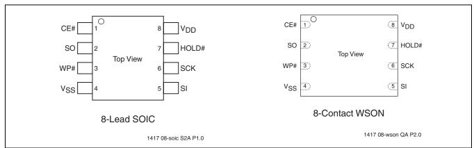
FIGURE 2: Pin Assignments
