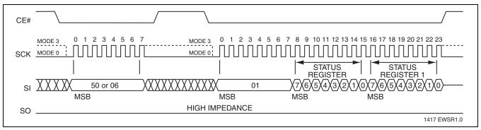
FIGURE 21: Enable-Write-Status-Register (EWSR) or
