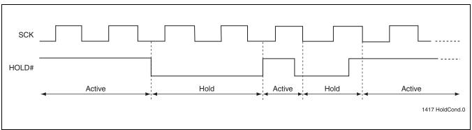
FIGURE 4: Hold Condition Waveform
