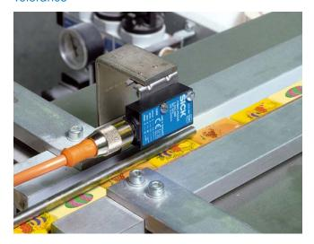
Tolerances can be easily configured for color sensors, ranging from coarse to fine depending on the application.
