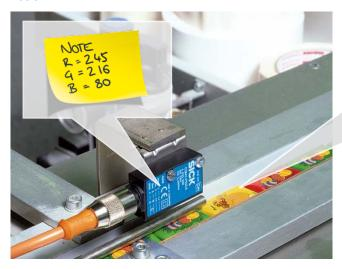
Reference colors can be easily stored via the teach-in procedure. If the color sensor detects the stored value, it automatically activates the switching output.
