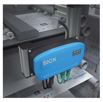
The RS25 register sensor is impressively simple and quick to use and features automatic teach-in mechanisms. This reduces machine setup and conversion times. It consists of a sensor head, fibers, and evaluation unit. Using an RGB light ensures excellent reading quality.
