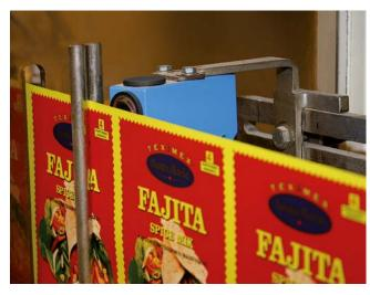
The size of the color sensor's light spot depends on the sensing distance.
