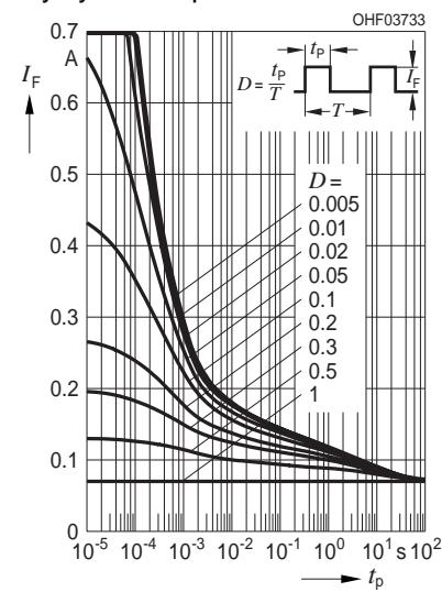
**Permissible Pulse Handling Capability  $I_F = f(\tau)$**  $T_A = 85^\circ\text{C}$ , duty cycle  $D = \text{parameter}$
