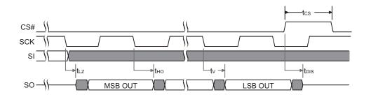
Figure 4.10 SPI MIO Timing
