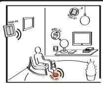
Radio foot transmitter RNL-01 controls operation of RWL-01 radio lighting switch (switch on / switch off) or RDP-01 radio dimmer (switch on / switch off, light brightening / dimming). The receivers can be controlled by 4-channel button radio transmitter RNK-04. The RNL-02 transmitter does not require additional installation, external power supply connection and mounting.
