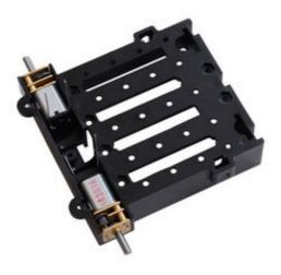
Zumo chassis being assembled with two micro metal gearmotors.
