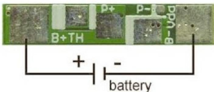
**Protection Circuit Module For 1S Li-ion/Li-polymer/LiFePO4 Battery Pack**
