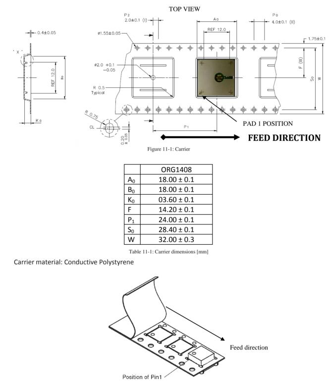
Figure 11-2: Module position
