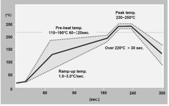
Figure 11-4: Recommended soldering profile
