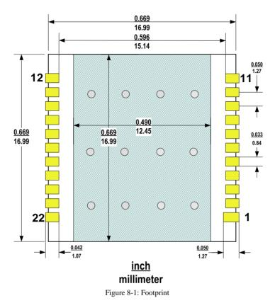
Ground pad at the middle should be connected to main Ground plane by multiple vias. Ground pad at the middle should be solder masked. Silk print of module's outline is highly recommended for SMT visual inspection.
