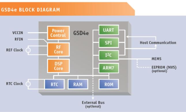
Figure 2-2: GSD4e functional block diagram
