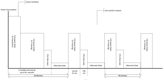
Figure 5-2: PTF<sup>™</sup> timing
