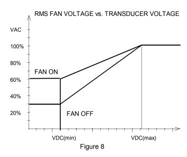
Fan On / Fan Off Feature (switch #1): To turn fans off automatically when transducer voltage drops below VDC (min), set switch #1 to the ON position. To keep fans running at idle speed below the VDC(min), set switch #1 to the OFF position. See figure 8.
