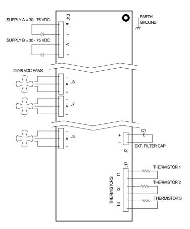
**FIGURE 1.0**: Connection diagram showing input power, fan, filter capacitor and temperature sensor connections for a Multi-SR configured for Temperature Sensor Based Fan Control.
