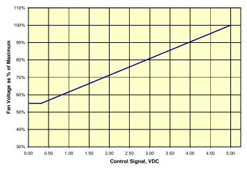
Chart 2.0: Fan voltage vs. control signal input.
