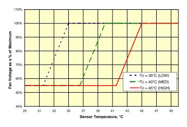
**Chart 1.0:** Fan voltage vs. sensor temperature for each control temperature setting.
