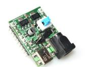
**NOTE!** Connection of two voltage sources may damage the circuit. When connecting the USB cable, please disconnect the DC cable and vice versa.
