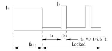
3rd wire signal Run : Square Wave Locked :  $V_{\text{H}}$  or  $V_{\text{L}}$
