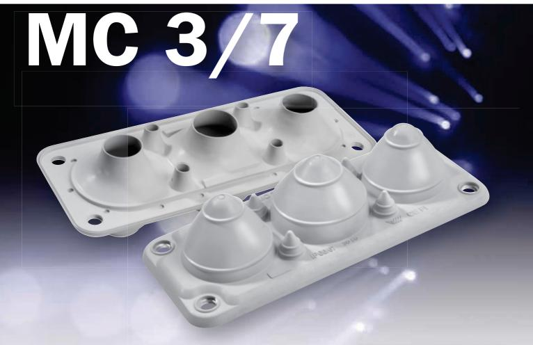
MC 3/7 Multigate is suitable for leading through both low and medium power current cables as well as various types of tubing. It fits directly to a C-standard cut-out (or FL 21).
