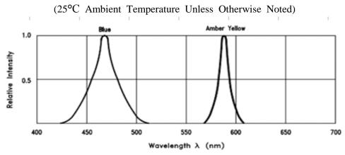
Fig.1 Relative Intensity vs. Wavelength
