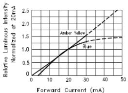
Fig.4 Relative Luminous Intensity vs. Forward Current
