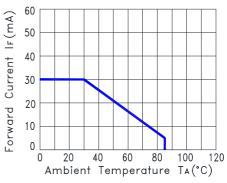
Fig.2 Forward Current Derating Curve
