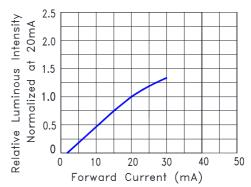
Fig.4 Relative Luminous Intensity vs. Forward Current
