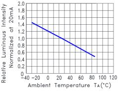
Fig.5 Relative Luminous Intensity VS. Ambient Temperature
