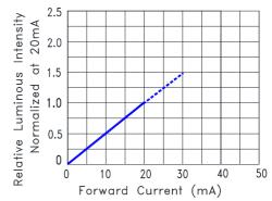
Fig.4 Relative Luminous Intensity vs. Forward Current
