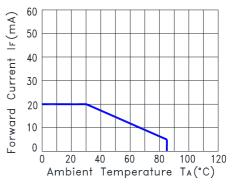
Fig.2 Forward Current Derating Curve
